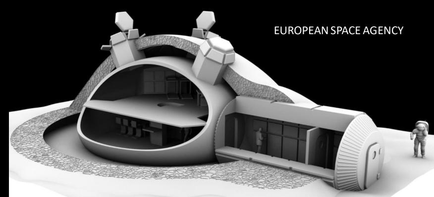
Exterior – Puncture-resistant combination of Nextel and Kevlar with reflective coating to mitigate against UV rays.
