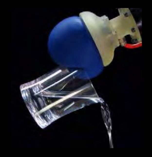
Internal gas bladder is an alt method of constricting the sheathed regolith so the granules interlock.
