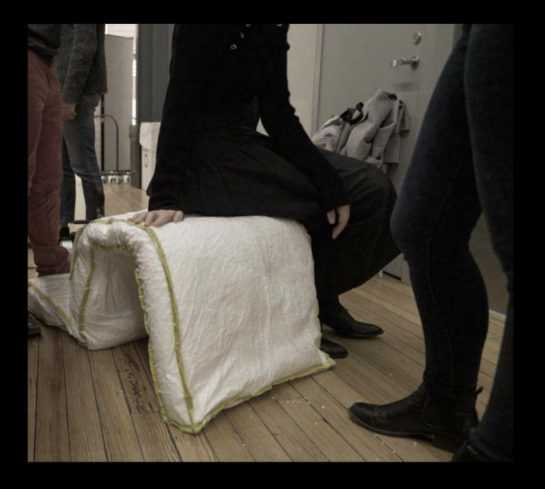
An airtight form was filled with bean-bag beads, then the air was vacuumed out.
